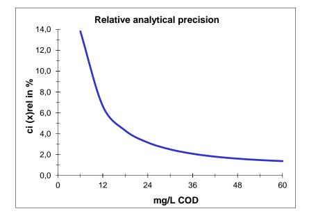
The technical data for cuvette test LCK1414 were determined in conformity with ISO 8466-1 and DIN 38402 A51 "Calibration of analysis methods".
